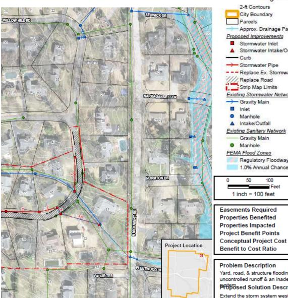
Approx. Drainage Path Proposed Improvements Stormwater Inlet Stormwater Intake/Outfall Replace Ex. Stormwater Line Replace Road Strip Map Limits Existing Stormwater Network ---- Gravity Main Manhole Intake/Outfall Existing Sanitary Network Gravity Main FEMA Flood Zones Regulatory Floodway 1.0% Annual Chance Flood Hazard 100 Feet 1 inch = 100 feet Easements Required Properties Benefited Properties Impacted Project Benefit Points 630.00 \$1,497,974.06
